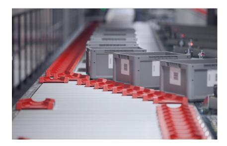
As soon as an order is finished, it is taken out of the backside of the racking, after which it is transported to separate packing workstations where 280 packers make the goods ready for shipping. Cartons ready to be shipped travel to the outbound chutes over the main conveying line. The cartons will be sorted using the shoe sorter (a high speed, very precise sortation technology) to its chute for outbound.
