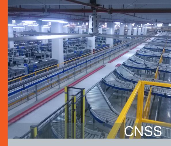
Put-to-Wall and mechanization system
